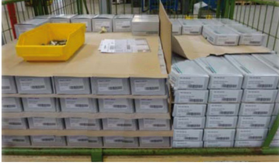
Mixed pallet with strong cardboard dividers
